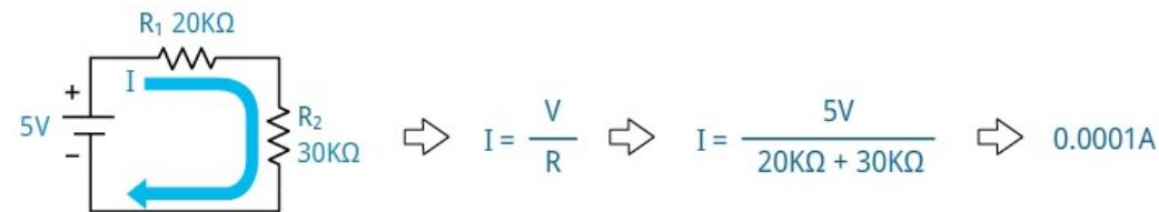
$$V_2 = I \times R_2 \Rightarrow V_2 = \frac{V_{CC}}{R_1 + R_2} \times R_2 \Rightarrow V_2 = V_{CC} \times \frac{R_2}{R_1 + R_2}$$
